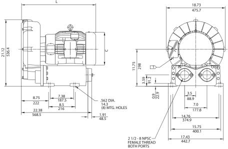
MODEL L (IN/MM) 1) TERMINAL BOX CONNECTOR HOLE 1.06 (26.9) DIA.
